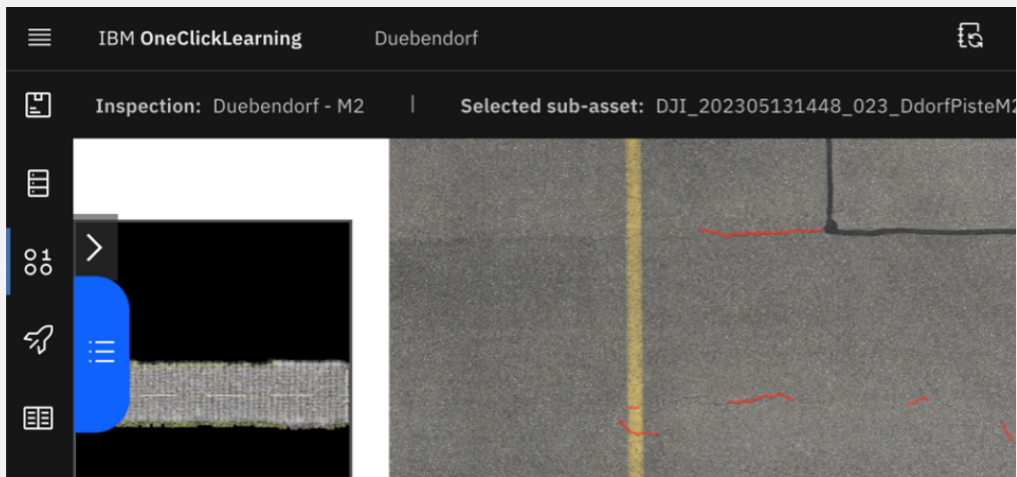
Figure 9: OCL image viewer on which crack detections are marked in red on the original image.
