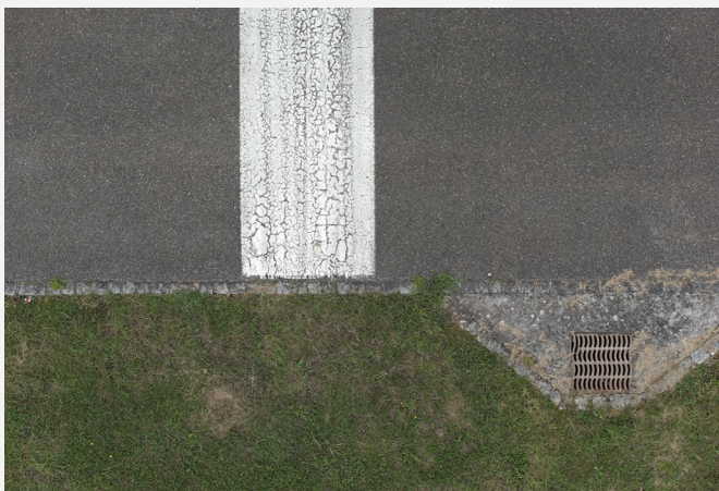
Figure 3: Representative sample of the originally captured images of M2. The image resolution is 0.75 mm/pixel. The GSD of M2 is three times larger than that of M1. This becomes apparent from the approximately nine times larger area covered by the M2 reference image compared to M1.
